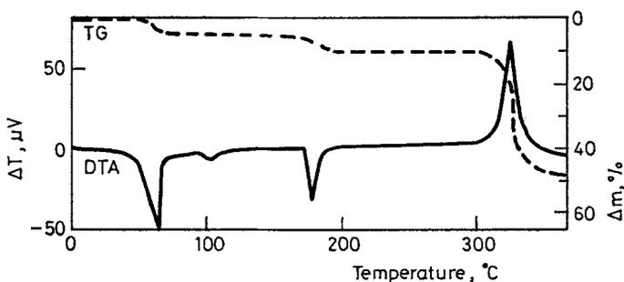
Fig. 3 Simultaneous TG and DTA for mixed cerium-50 mol% gadolinium oxalate at a heating rate of 5 deg/min
