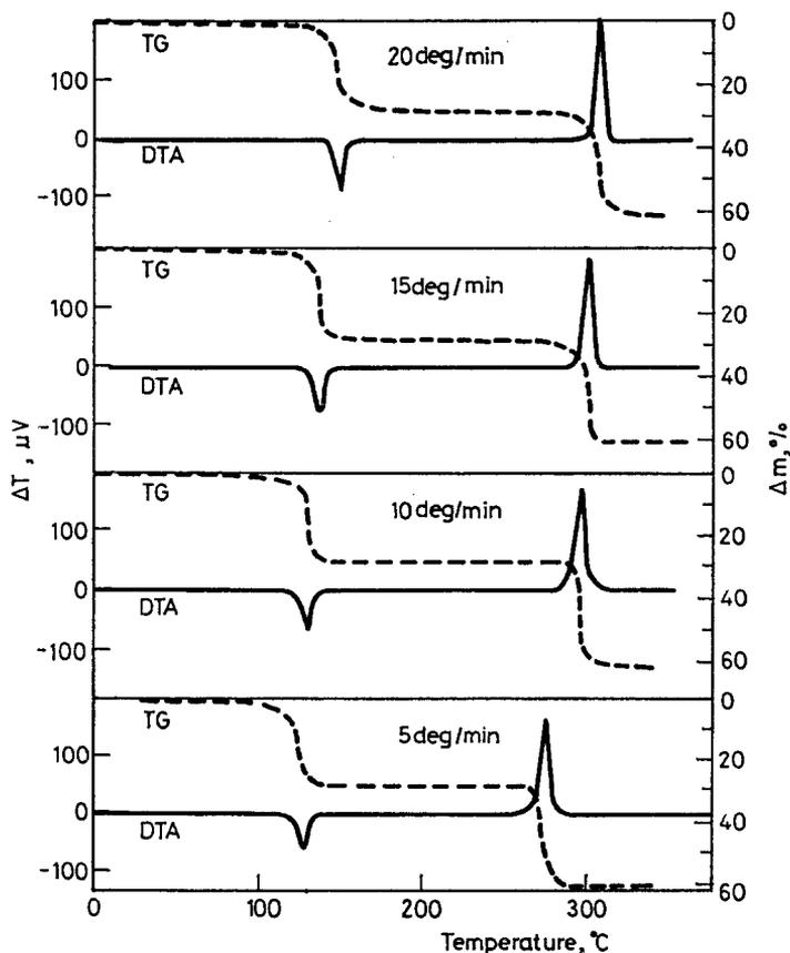
Fig. 1 Simultaneous TG and DTA for cerous oxalate at different heating rates
