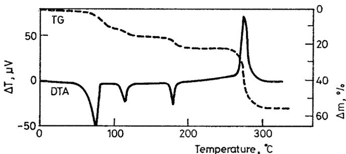
Fig. 2 Simultaneous TG and DTA for mixed cerium-20 mol% gadolinium oxalates at a heating rate of 5 deg/min
