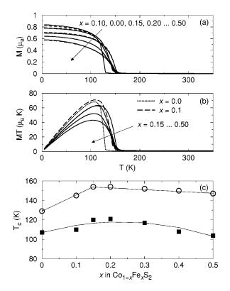
FIG. 3. (a) Zero-field cooled (dashed lines) and field-cooled magnetization as a function of temperature of the  $\text{Co}_{1-x}\text{Fe}_x\text{S}_2$  samples. (b) Field-cooled *MT* vs *T*. (c)  $T_c$  onset (circles) and midpoint, corresponding to the maximum value (squares) obtained from the *MT* vs *T* plot, as a function of *x*. The lines are guides to the eye.
