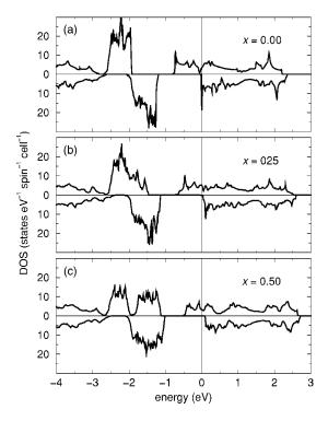
FIG. 6. Evolution of total LMTO densities of state as a function in x in  $\text{Co}_{1-x}\text{Fe}_x\text{S}_2$ : (a)  $\text{CoS}_2$  (x=0.00), (b)  $\text{Co}_{0.75}\text{Fe}_{0.25}\text{S}_2$  (x =0.25), and (c)  $\text{Co}_{0.50}\text{Fe}_{0.50}\text{S}_2$  (x=0.50).
