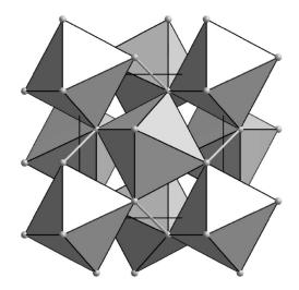
FIG. 1. MX<sub>2</sub> pyrite crystal structure showing MX<sub>6</sub> octahedra corner connected through X atoms which, in addition, are bonded (shown by sticks) to X atoms on neighboring octahedra. The coordination of X is 3(M)+1(X). X<sub>2</sub> sticks and M atoms (at the centers of the octahedra) form two interpenetrating fcc lattices and a structure related to NaCl.
