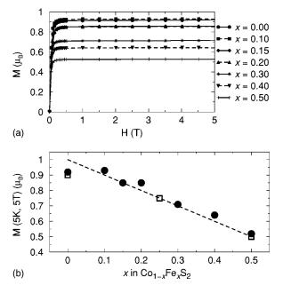
FIG. 4. (a) Magnetization at 5 K as a function of field. Since none of the samples show appreciable hysteresis, only the positive quadrant is displayed. Data were acquired from 5 T through 0 T. (b) Closed circles are measured saturation magnetization (5 K, 5 T) as a function of x. The open squares are the calculated LMTO magnetic moments. The dashed line is the expected spin only value assuming every  $e_g$  electron contributes 1  $\mu_B$ .
