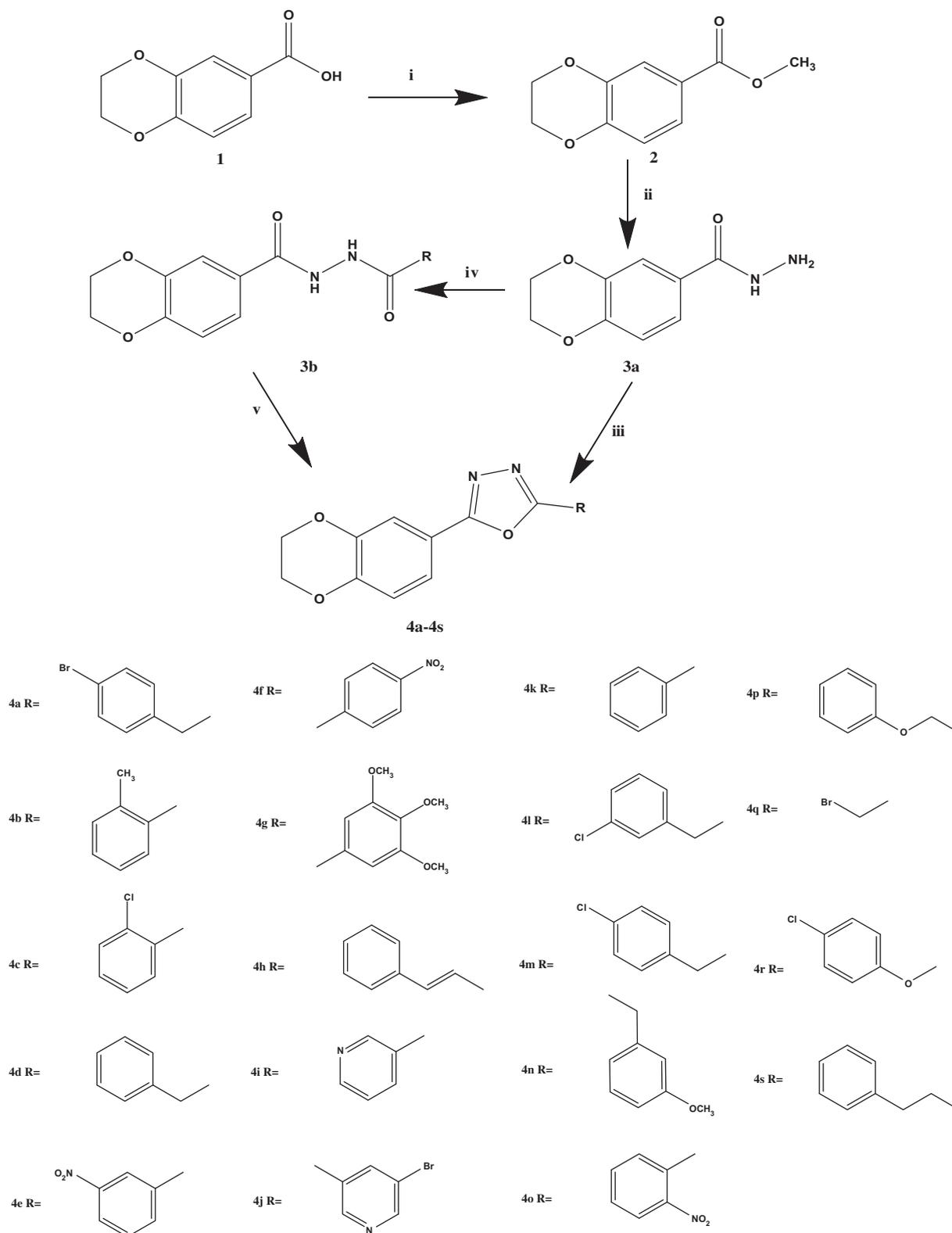
**Scheme 1.** General synthesis of compounds **4a–4s**. Reagents and conditions: (i) methanol, concentrated sulfuric acid; 90 °C; (ii)  $\text{NH}_2\text{NH}_2 \cdot \text{H}_2\text{O}$ , ethanol; 90 °C; (iii) aliphatic or aromatic carboxylic acids,  $\text{POCl}_3$ ; 110 °C; (iv) EDC·HCl, HOBT, dichloromethane, rt; (v)  $\text{POCl}_3$ ; 100 °C.
