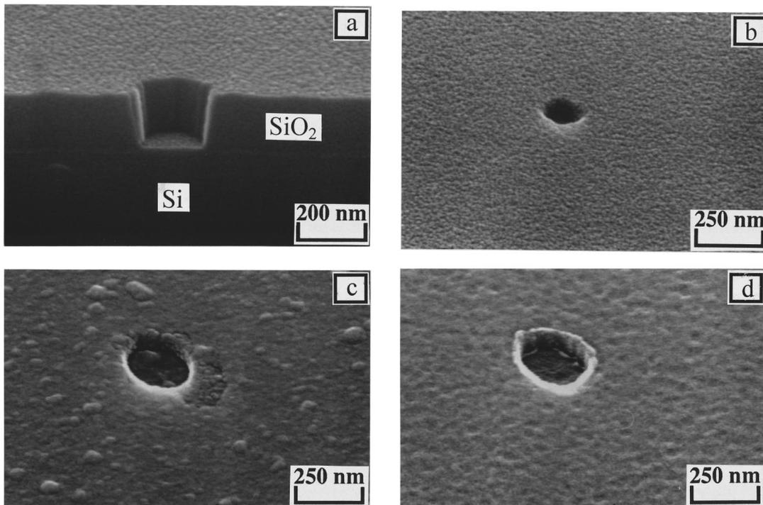
FIG. 3. SEM images of (a) a  $0.18 \mu m$  contact hole, cross-section, (b) as-deposited Co film on the SEG Si layer inside a  $0.13 \mu m$  contact hole, (c)  $CoSi_2$  formed on the SEG Si layer inside a  $0.2 \mu m$  contact hole after RTA treatment at 700 °C, (d) selectively etched  $CoSi_2$  film on the SEG Si layer inside a  $0.23 \mu m$  contact hole after RTA treatment at 700 °C.
