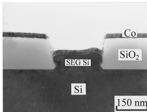
FIG. 1. Cross-section TEM image (taken along the [110] direction) of the as-deposited Co film on SEG Si layer inside 0.2 μm linear oxide opening.
