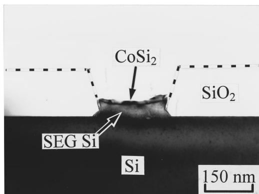
FIG. 4. Cross-section TEM image of the  $\text{CoSi}_2$  film on the SEG Si layer inside a  $0.23 \mu\text{m}$  linear opening after RTA at  $700^\circ\text{C}$  and selective etching treatment.
