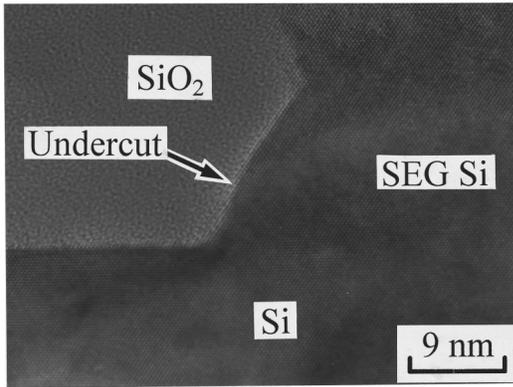
FIG. 2. HRTEM image of the interfaces between SEG Si and Si substrate as well as the oxide sidewall.
