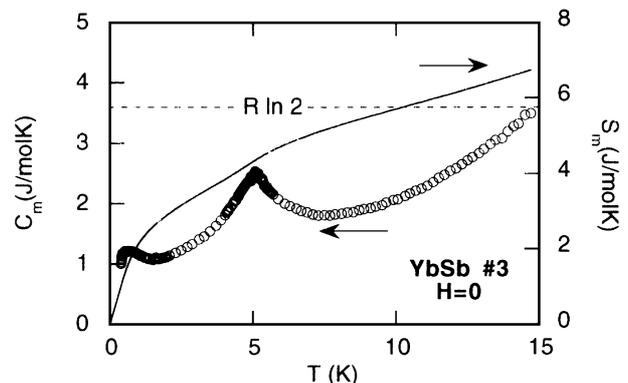
Fig. 2. Temperature dependence of the magnetic specific heat and magnetic entropy for YbSb under zero magnetic field.
