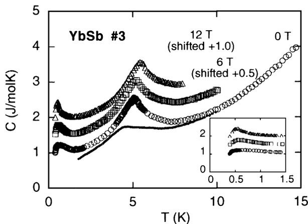
Fig. 1. Temperature dependence of the specific heat for YbSb #3 under external magnetic fields of 0, 6 and 12 T, respectively. Inset shows the lower temperature region. It should be noted that the values of the specific heat for 6 T and 12 T are shifted by +0.5 and +1.0, respectively. The solid line shows the result of a previous study on YbSb #1 under zero magnetic field.<sup>8)</sup>
