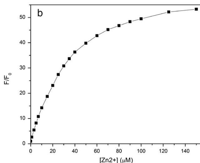
**Fig. 2.** (a) Fluorescence spectra of Sensor Zn (25  $\mu\text{M}$ ,  $\lambda_{\text{ex}} = 470 \text{ nm}$ ) in HEPES buffer (20 mM, pH = 7.4) in the presence of different concentration of  $\text{Zn}^{2+}$ . (b) The corresponding  $\text{Zn}^{2+}$  titration profile of the emission at 550 nm.
