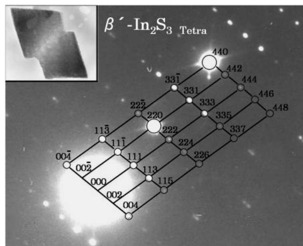
Fig. 5. TEM and ED images of the coalesced particle of two octahedral particles with parallel relationship. The super-diffraction spots can be indexed as those of the  $\beta'$  phase.
