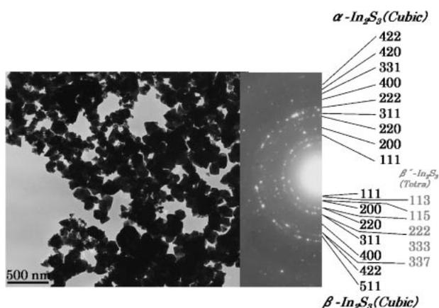
Fig. 3. TEM image of collected particles and corresponding electron diffraction pattern. The electron diffraction rings indicate the growth of three polytypes.
