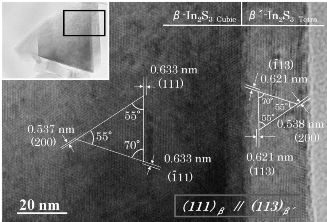
Fig. 6. Two-phase particle of  $\beta$  and  $\beta'$  phases. The  $\beta'$  phase grew on the  $\beta$  phase with the parallel relationship of  $(111)_{\beta} \parallel (113)_{\beta'}$ .
