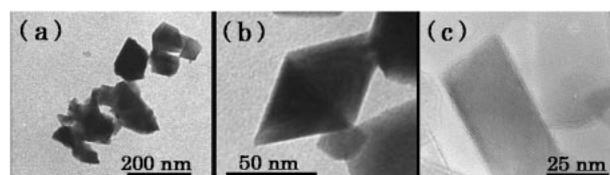
Fig. 2. (a)  $\alpha$ , (b)  $\beta$  and (c)  $\beta'$  of  $\text{In}_2\text{S}_3$  phases electron microscopic images of typical  $\text{In}_2\text{S}_3$  particles. The difference in the morphology reflects the structural difference.
