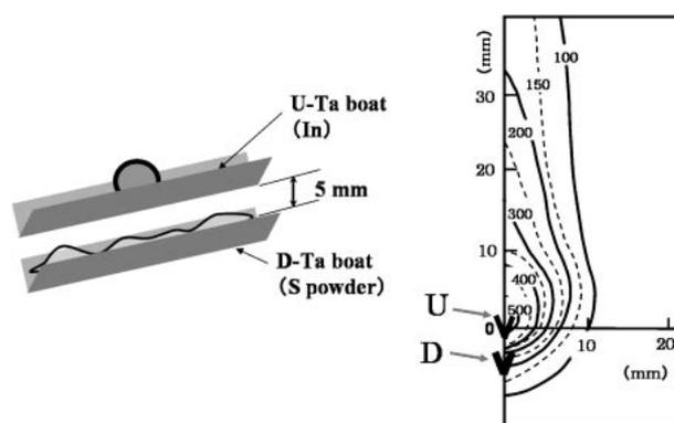
Fig. 1. Schematic of the set up for producing the sulfide particle by making use of the temperature distribution and convection flow in smoke. This method is called the advanced gas evaporation method (AGEM).
