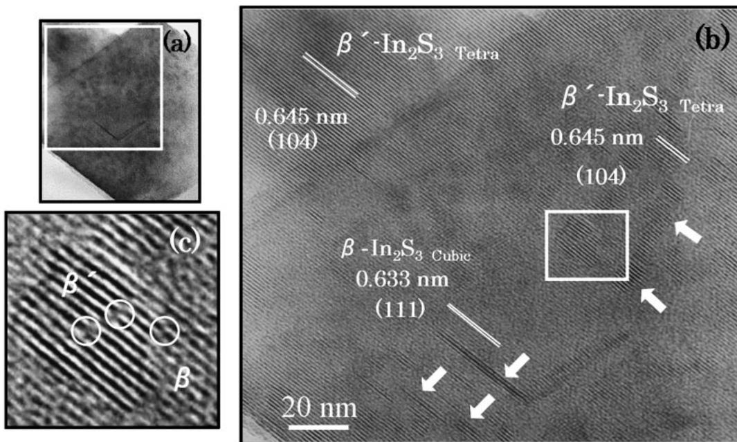
Fig. 7. HREM image of octahedral particle. The G.P. contrast and misfit dislocations are seen with the coexistence of two phases.
