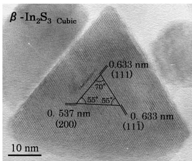
Fig. 4. HRTEM image of a particle. The lattice distance and crossed angles indicate the growth of the  $\beta$  phase.
