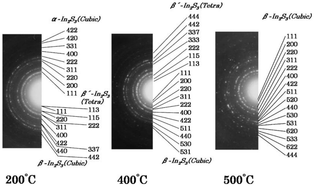
Fig. 8. ED patterns of the heat-treated collected samples. Phase transition temperatures of  $\alpha$ ,  $\beta$  and  $\beta'$  were determined. The  $\alpha$  phase disappeared at 400°C. The  $\beta'$  transformed to the  $\beta$  phase at 500°C.
