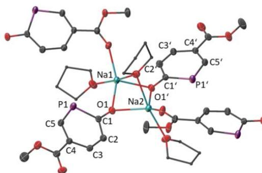
**Figure 5.** X-ray solid state structure of **8**. Ellipsoids are drawn at the 50% probability level. Selected bond parameters in [Å] and [°]: P1-C1 1.792(1); C1-C2 1.435(2); C2-C3 1.379(2); C3-C4 1.407(2); C4-C5 1.395(2); C5-P1 1.724(1); C1-O1 1.277(1); C5-P1-C1 101.79(5); P1-C1-C2 120.78(8); C4-C5-P1 126.70(8).
