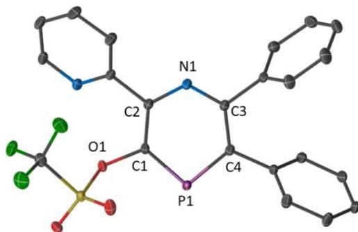
**Figure 3.** X-ray solid state structure of **4c**. Ellipsoids are drawn at the 50% probability level. Selected bond parameters in [Å] and [°]: P1-C1 1.732(2); C1-C2 1.399(2); C2-N1 1.345(2); N1-C3 1.339(2); C3-C4 1.411(2); C4-P1 1.733(2); C1-O1 1.436(2); C4-P1-C1 98.70(7); P1-C1-C2 127.2(1); C1-C2-N1; C3-C4-P1 123.2(1).
