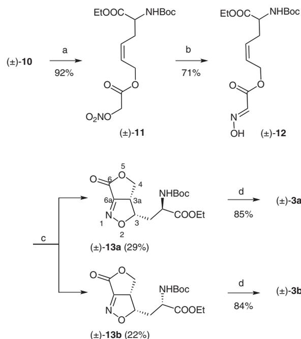
**Scheme 3** Reagents and conditions: (a) AgNO<sub>3</sub>, MeCN; (b) NH<sub>2</sub>OH·HCl, NaOAc, DMSO; (c) NaOCl (3.5%), CH<sub>2</sub>Cl<sub>2</sub>; (d) K<sub>2</sub>CO<sub>3</sub>, EtOH.
