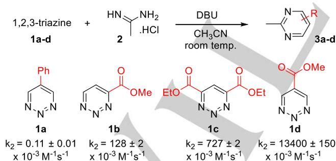
**Scheme 3.** Scheme showing conditions used during measurements of reaction kinetics. The determined second order rate constants for individual 1,2,3-triazines are depicted below the structures.
