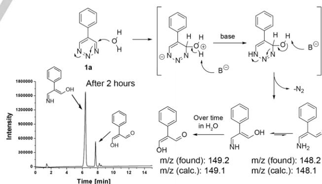
**Scheme 2.** Proposed reaction mechanism leading to formation of side products from **1a** in CH<sub>3</sub>CN/H<sub>2</sub>O in the presence of the base. Bottom left is the HPLC chromatogram showing product distribution after 2 hours.
