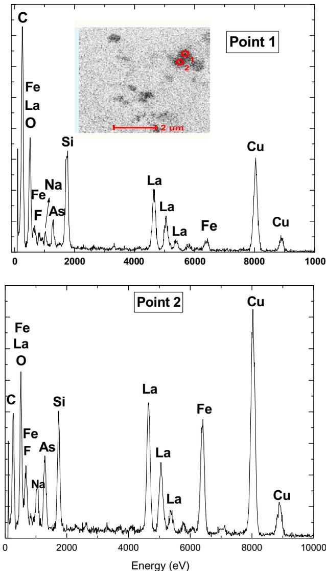
**Fig. 2.** EDX spectra from two microcrystals of  $\text{La}_{0.85}\text{Na}_{0.15}\text{O}_{0.85}\text{F}_{0.15}\text{FeAs}$  compound. The inset shows the scanning transmission electron microscopy (STEM) image. Carbon coated copper grid is responsible for the presence of Cu and C peaks in EDX spectra while Si is due to detector of microscope.
