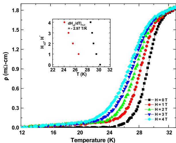
**Fig. 4.** Temperature dependence of the electrical resistivity of  $\text{La}_{0.85}\text{Na}_{0.15}\text{O}_{0.85}\text{F}_{0.15}\text{FeAs}$  under different magnetic fields. Inset shows the temperature dependence of estimated upper critical field (■) and irreversibility field (●).
