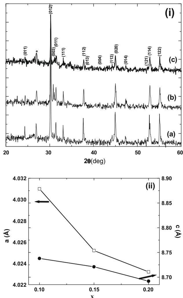
Fig. 1. (i) Powder X-ray diffraction patterns (PXRD) of (a)  $\text{La}_{0.9}\text{Na}_{0.1}\text{O}_{0.9}\text{F}_{0.1}\text{FeAs}$  (b)  $\text{La}_{0.85}\text{Na}_{0.15}\text{O}_{0.85}\text{F}_{0.15}\text{FeAs}$  and (c)  $\text{La}_{0.8}\text{Na}_{0.2}\text{O}_{0.8}\text{F}_{0.2}\text{FeAs}$  sintered at  $1080^\circ\text{C}$ . The impurity phase is  $\text{LaOF}$  (\*). (ii) Variation of lattice parameters with doping for  $\text{La}_{1-x}\text{Na}_x\text{O}_{1-x}\text{F}_x\text{FeAs}$ .
