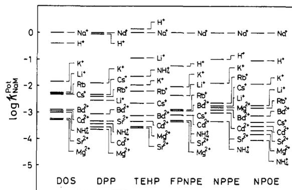
**Figure 1.** Selectivity coefficients for  $\text{Na}^+$  in electrodes of calixaryl decyl ester 1 with different membrane solvents. For details see Experimental Section.
