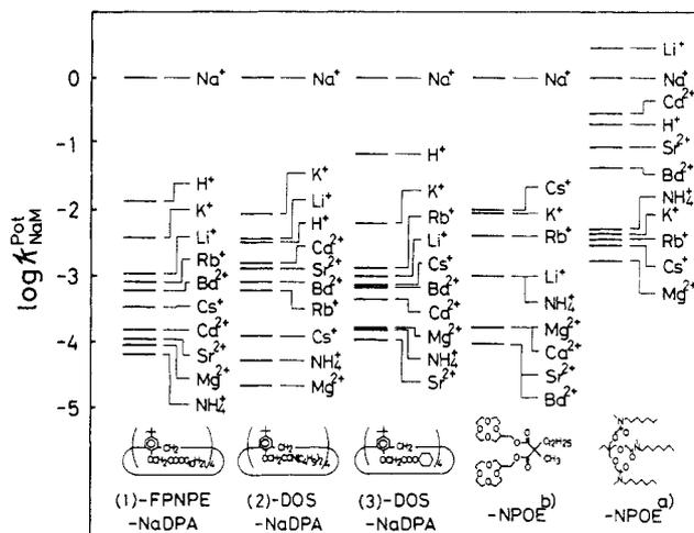
**Figure 5.** Selectivity comparison among  $\text{Na}^+$ -selective electrodes of lipophilic calixarene neutral carriers **1-3** and previous neutral-carrier-type PVC membrane  $\text{Na}^+$  electrodes: (a) ref 1; (b) ref 4.
