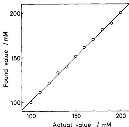
**Figure 7.** Correlation of actual values of  $\text{Na}^+$  concentrations in control sera and those found with 1-based  $\text{Na}^+$  electrode. For details see Experimental Section.
