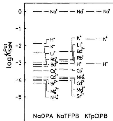
**Figure 4.** Selectivity coefficients for  $\text{Na}^+$  in electrodes of 1/FPNPE membrane containing different lipophilic salts. The membrane composition is identical with that for the optimized membrane.
