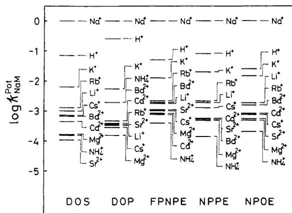
**Figure 3.** Selectivity coefficients for  $\text{Na}^+$  in electrodes of calixaryl cyclohexyl ester **3** with different membrane solvents.
