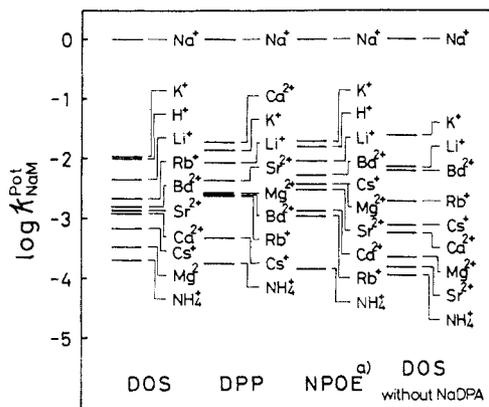
**Figure 2.** Selectivity coefficients for  $\text{Na}^+$  in electrodes of calixaryl dibutylamide **2** with different membrane solvents, (a) apparent values.
