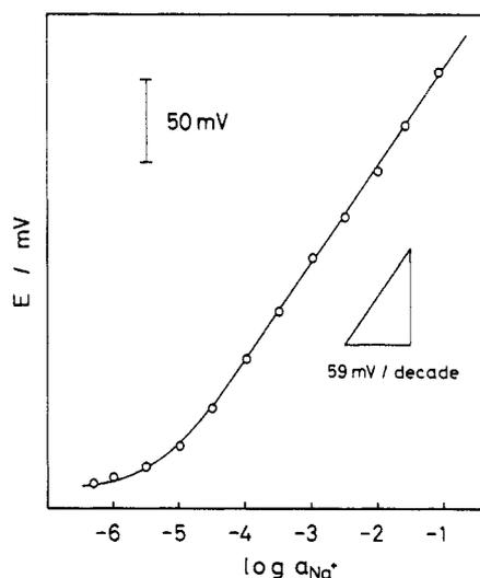
**Figure 6.** Calibration graph for  $\text{Na}^+$ -selective electrode with optimized 1/FPNPE membrane.
