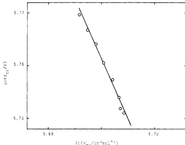
Figure 4. log-log plots of the molar volume at the transition points and the transition temperature for 8CB.
