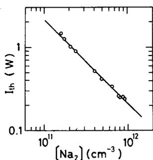
FIG. 2. Threshold Ar\* laser power  $I_{th}$  for particle formation as a function of Na<sub>2</sub> density [Na<sub>2</sub>].
