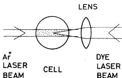
FIG. 4. Sketch showing the observed dissociation of NaH particles produced by  $\text{Ar}^+$  laser beam in the region where the dye laser beam tuned at the  $D_1$  line is applied.
