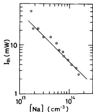
FIG. 3. Threshold power  $I_{th}$  of the dye laser tuned at the  $D_1$  line for particle formation as a function of Na density  $[\text{Na}]$ .
