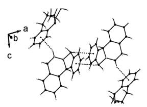
**Figure 5.** Part of the crystal structure of **5a**, showing the formation of the C—H $\cdots \pi$  intermolecular interactions built from C8—H8 $\cdots Cg1$  [symmetry code: 1-x, -y, 1-z] and C6—H6B $\cdots Cg2$  [symmetry code: x, 1/2-y, -1/2+z]. Dashed lines represent intermolecular interactions.
