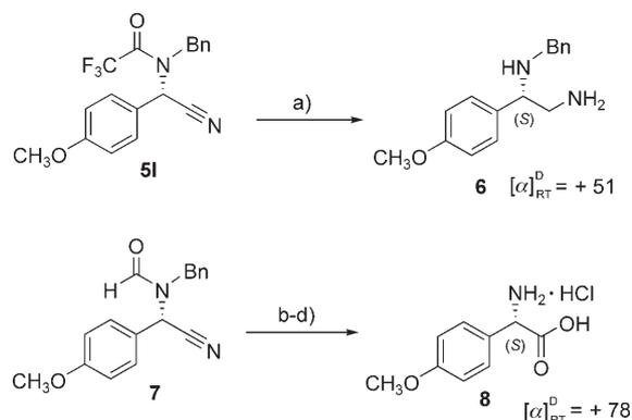
**Scheme 2.** Reduction and hydrolysis of amino nitriles **5I** and **7**. a) LiAlH<sub>4</sub>, Et<sub>2</sub>O; b) 65% (w/v) H<sub>2</sub>SO<sub>4</sub>, 45 °C, 20 h; c) HCl (conc.), 70 °C, 12 h; d) H<sub>2</sub>/Pd-C, MeOH.
