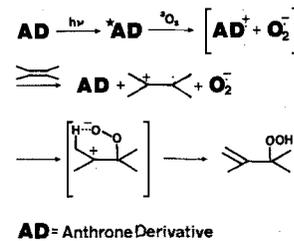
Fig. 6: Electron transfer photooxygenation of 2,3-dimethyl-2-butene
