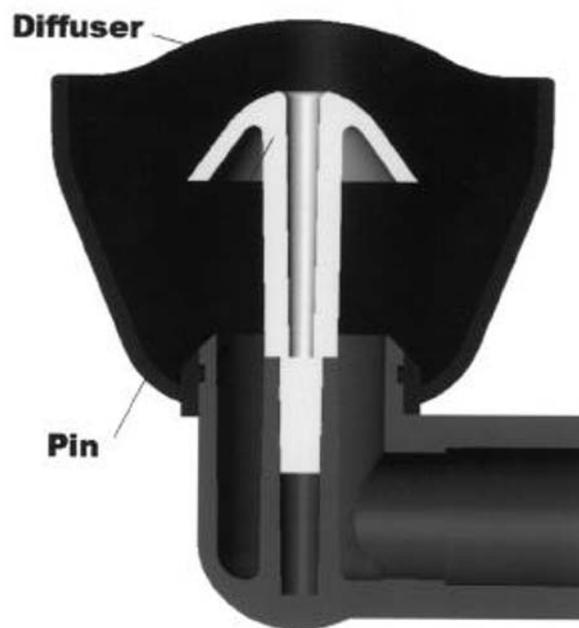
FIGURE 1 Cross-sectional drawing illustrating shape of the cup that houses the pin diffuser unique to the OxyArm™.
