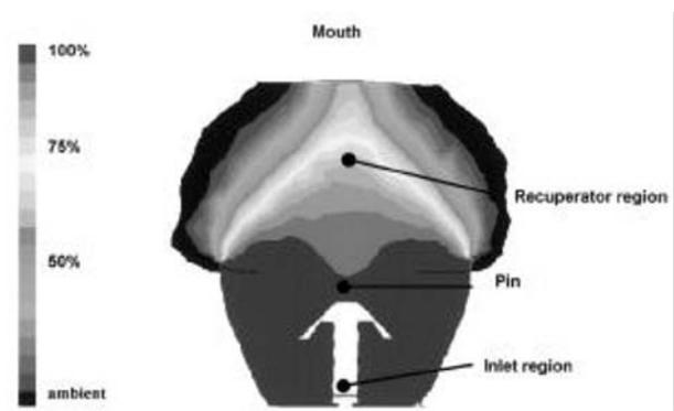
FIGURE 4 Oxygen ( $O_2$ ) mass fraction gradient of the OxyArm™ at  $4 \text{ L}\cdot\text{min}^{-1}$  with inspiration from computer simulated wind tunnel testing. The shape of the diffuser (recuperator region) causes velocity vortices to develop which concentrate the flow of  $O_2$  from the pin into a flame-like shape towards the face.
