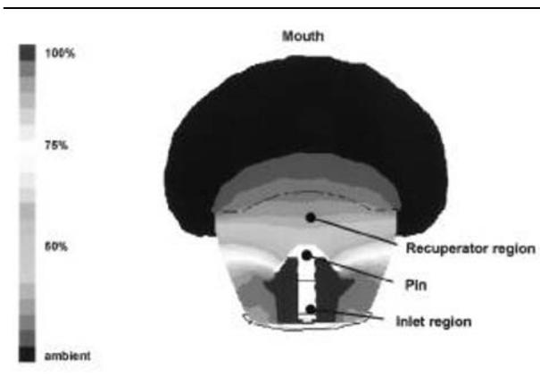
FIGURE 3 Oxygen ( $O_2$ ) mass fraction gradient of the OxyArm™ at  $4 \text{ L}\cdot\text{min}^{-1}$  from computer simulated wind tunnel testing.  $O_2$  diffuses out from the inlet region out from the pin like a mushroom cloud towards the face in passive conditions (no inspiration). The recuperator region is the concave area of the diffuser cup.
