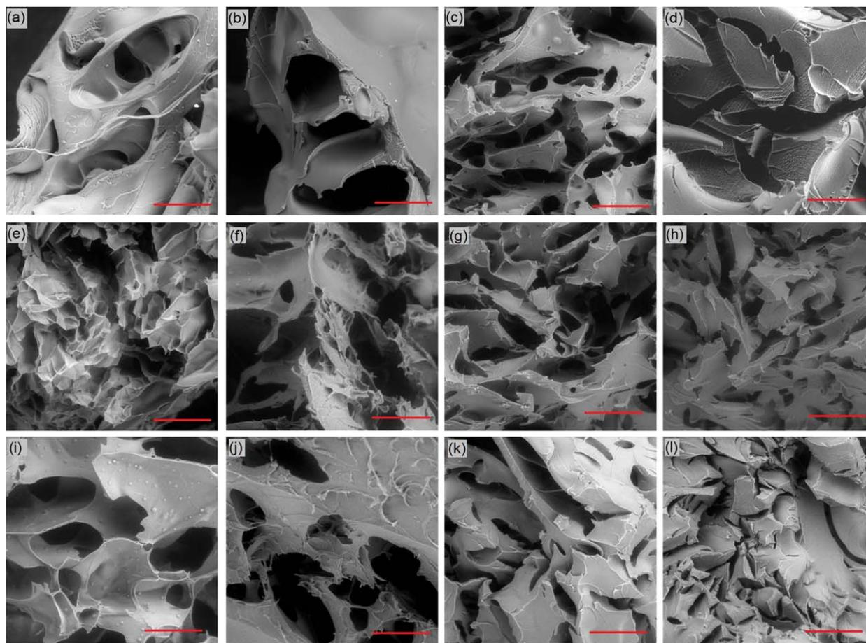
**FIGURE 3** SEM micrographs of the morphology of freeze-dried samples. **ButBisOx** (a)–(d), **HexBisOx** (e)–(h), **OctBisOx** (i)–(l), percentage of crosslinker: 2% column 1; 3% column 2; 5% column 3; 10% column 4; scale bar 200  $\mu\text{m}$ . [Color figure can be viewed in the online issue, which is available at [wileyonlinelibrary.com](http://wileyonlinelibrary.com).]
