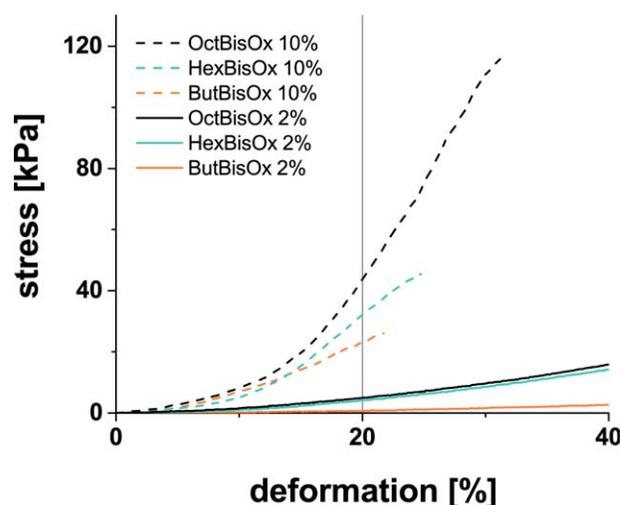
**FIGURE 6** Representative stress-deformation curves of **ButBisOx** (orange), **HexBisOx** (blue), and **OctBisOx** (black) hydrogels containing 2% (solid) and 10% (dashed) of crosslinker. [Color figure can be viewed in the online issue, which is available at [wileyonlinelibrary.com](http://wileyonlinelibrary.com).]
