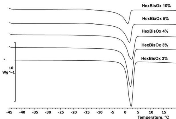
**FIGURE 5** The representative DSC heating curves for **HexBisOx** hydrogel with different crosslinker percentage.
