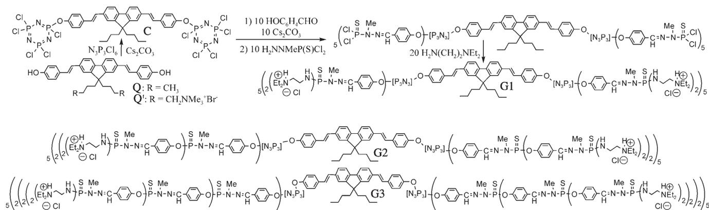
**Scheme 2.** Synthesis of **G1** from **Q**, and structures of **G2** and **G3**. The core reagent **C** was prepared from the bisphenol quadrupolar chromophore **Q** by treatment with  $\text{N}_3\text{P}_3\text{Cl}_6$  under basic conditions.
