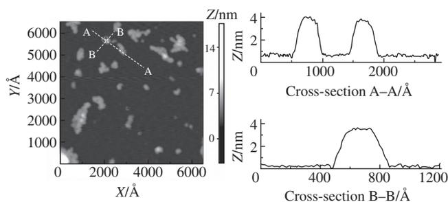
**Figure 2** AFM image of the aggregates of triantennary glycopeptide (*n* = 7); solution of the glycopeptide (1 mg cm<sup>-3</sup>) was placed on mica surface, kept for 1 min and then unadsorbed material was removed by a nitrogen stream.
