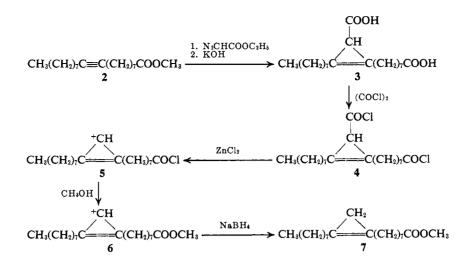
ride, and zinc chloride were all found to be effective in such decarbonylations, we eventually settled on zinc chloride as the reagent of choice for the conversion of  $4 \text{ to } 5.^{16}$
