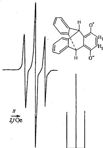
Fig. 1. EPR spectrum of triptycenesemiquinone anion produced by electrochemical reduction of quinone I in dimethylformamide.
