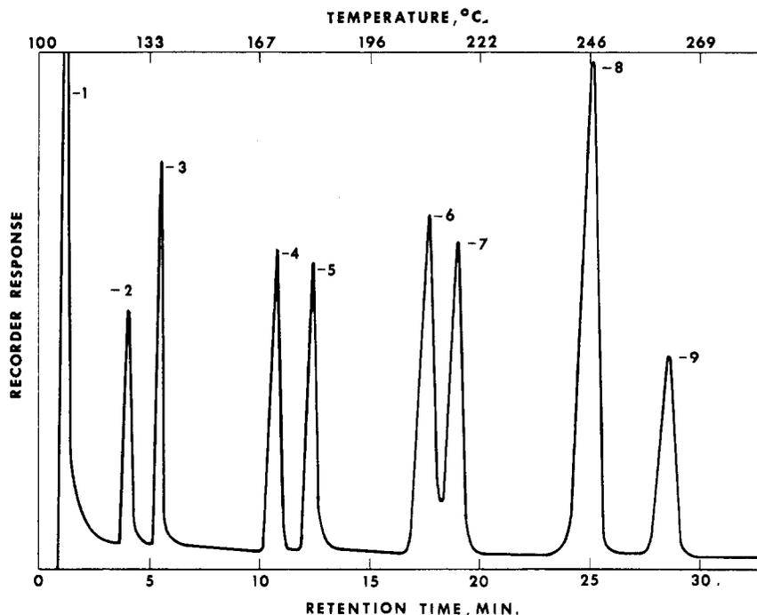
Figure 2. Identification of hydroxymethylphenol acetates, hemiformal-free
