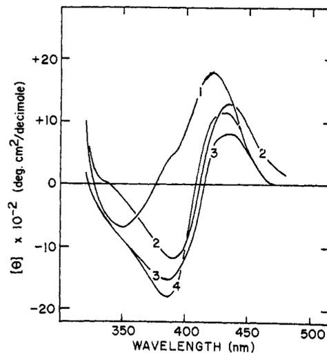
FIGURE 6: Molecular ellipticity of HNB-papain as a function of wavelength. Curve 1, mercuri-HNB-papain in Tris-acetate, pH 7.5; curve 2, activated HNB-papain in Tris-acetate, pH 7.5; curve 3, activated HNB-papain in phosphate, pH 7.5; curve 4, activated HNB-papain in phosphate, pH 7.5, 0.46 mM in  $\text{Bz-NHCH}_2\text{CN}$ .
