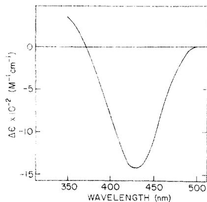
FIGURE 4: Iodoacetate-induced change in molar absorptivity of HNB-papain ( $56.1 \mu\text{M}$ ) at pH 7.5, as a function of wavelength.
