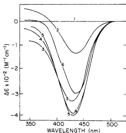
FIGURE 3: Differential molar absorptivities arising from interaction of activated HNB-papain ( $6.8 \times 10^{-5}$  M) at pH 7.5 with various concentrations of the competitive inhibitor, Bz-NHCH<sub>2</sub>CN. Curve 1, no inhibitor, is recorded as zero, and other curves are recorded relative to this value. Curve 2, 0.1 mM Bz-NHCH<sub>2</sub>CN; curve 3, 0.2 mM; curve 4, 0.5 mM; curve 5, 0.83 mM; curve 6, 1.0 mM.
