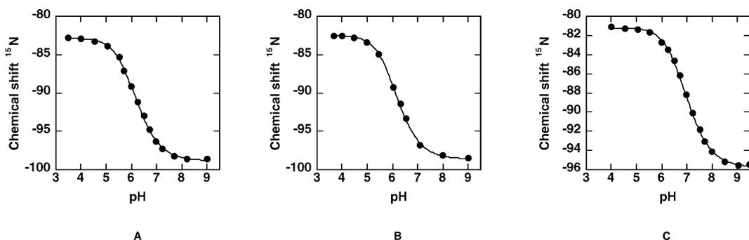
**Figure 2.** Determination of aminonucleoside  $pK_a$  values by following  $^{15}\text{N}$  NMR chemical shifts versus pH. (A)  $2'$ - $^{15}\text{N}$ -amino- $2'$ -deoxyadenosine,  $pK_a = 6.2$ ; (B)  $2'$ - $^{15}\text{N}$ -amino- $2'$ -deoxyguanosine,  $pK_a = 6.2$ ; (C)  $3'$ - $^{15}\text{N}$ -amino- $3'$ -deoxyguanosine,  $pK_a = 7.0$ . Data were fit according to eq 1.
