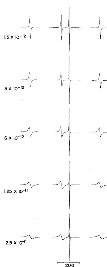
Figure 13. Calculated line shapes for the radical  $\dot{\text{C}}\text{F}_2\text{OSiEt}_3$  as a function of the rotational correlation time in sec (see text).
