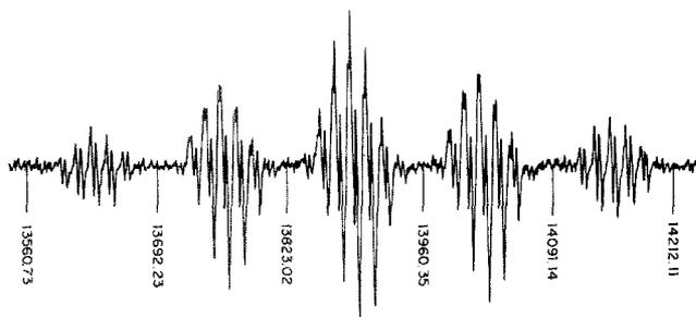
Figure 7. Esr spectrum of the radical  $(\text{CF}_3\text{CF}_2)_2\dot{\text{C}}\text{OH}$  obtained by photolysis of perfluoroethyl ketone in cyclopropane at  $-40^\circ$ .
