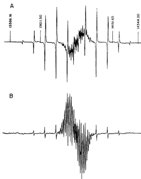
**Figure 5.** ESR spectra at high (A) and low microwave power levels (B) resulting by photolysis of a dilute solution of perfluoroisopropyl ketone in perfluoro-1,2-dimethylcyclobutane showing the spectra of the perfluoroisopropyl radical (doublet-of-septets) and of the adduct radical XIV (room temperature).
