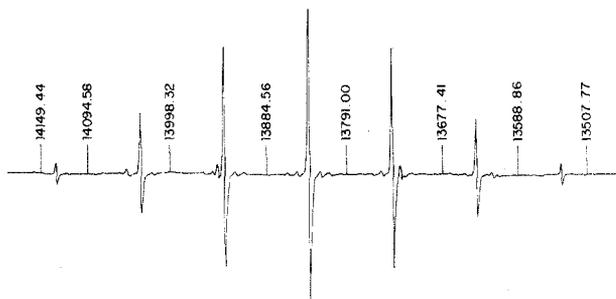
**Figure 9.** ESR spectrum (septet) of the  $(\text{CF}_3)_2\dot{\text{C}}\text{OSiEt}_3$  radical resulting by addition of triethylsilyl radicals to hexafluoroacetone at  $-40^\circ$  in a cyclopropane solution. Some of the minor peaks are due to hyperfine interaction with  $^{29}\text{Si}$ .
