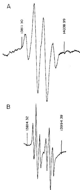
**Figure 6.** ESR spectra of the trifluoroacetyl radical (A,  $-97^\circ$ ) and of the perfluoropropionyl radical (B,  $-135^\circ$ ) obtained by photolysis of cyclopropane solutions containing di-*tert*-butyl peroxide and trifluoroacetaldehyde and pentafluoropropionaldehyde, respectively.
