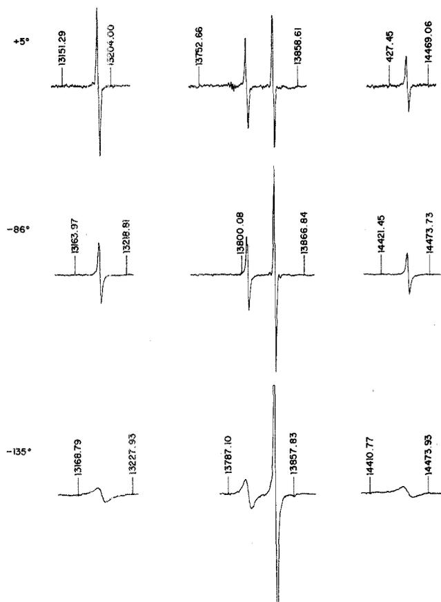
Figure 12. Temperature dependence of the line shapes in the esr spectrum of the  $\text{CF}_2\text{OSiEt}_3$  radical.
