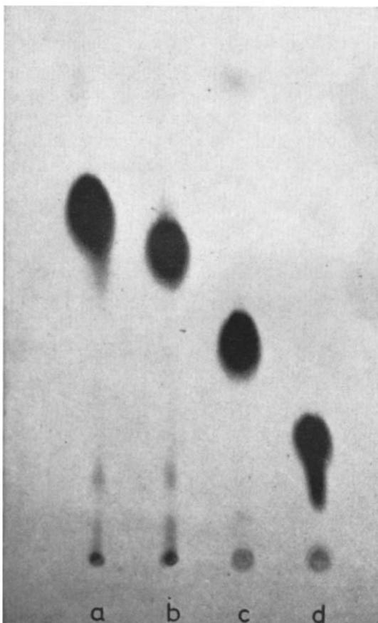
Fig. 1. Thin-layer chromatograms of neutral diol lipids. (a) 2-*trans*-octadec-1'-enyloxy-1-O-octadecanoyl-ethanol, (b) 2-*cis*-octadec-1'-enyloxy-1-O-octadecanoyl-ethanol, (c) 2-octadecyloxy-1-O-octadecanoyl-ethanol, (d) 1,2-di-O-octadecanoyl-ethanediol. Adsorbent: Silica Gel G. Solvent: hexane-diethyl ether (95/5, v/v).
