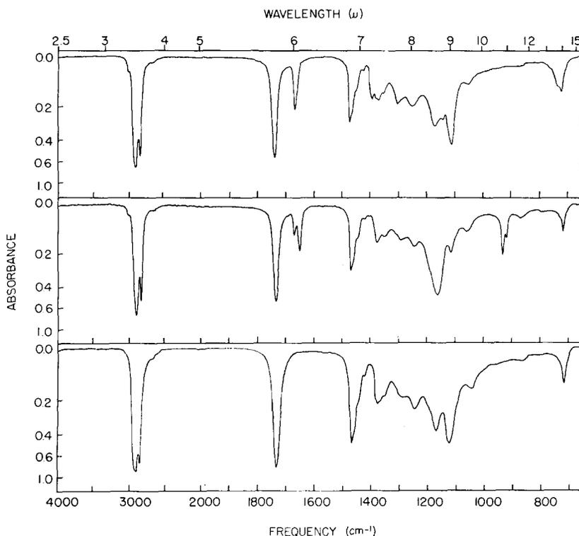
Fig. 3. Infrared spectra of 2-*cis*-octadec-1'-enyloxy-1-O-octadecanoyl-ethanol (top), 2-*trans*-octadec-1'-enyloxy-1-O-octadecanoyl-ethanol (center) and 2-octadecyloxy-1-O-octadecanoyl-ethanol (bottom).
