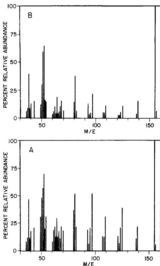
FIG. 3. Mass spectra of authentic nitrohydroquinone (A) and of the product formed microbially from *m*-nitrophenol (B).
