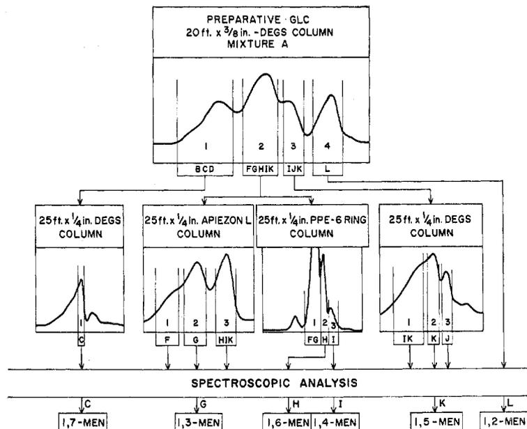
Figure 3. Chromatographic separations of Mixture A
