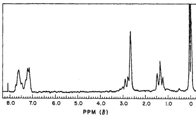
Figure 7. NMR spectrum of 1-methyl-7-ethylnaphthalene
