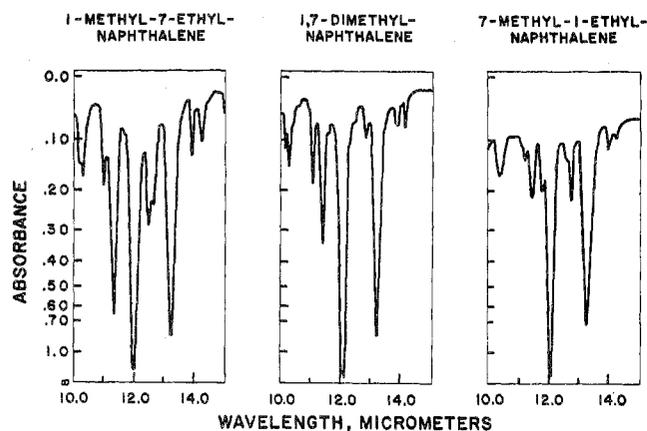
Figure 5. Infrared spectra (10- to 15-micrometer region) of three [1,7] disubstituted alkylnaphthalenes
