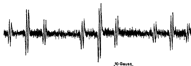
FIGURE 3 The e.s.r. spectrum of the pentafluorophenoxymethyl radical
