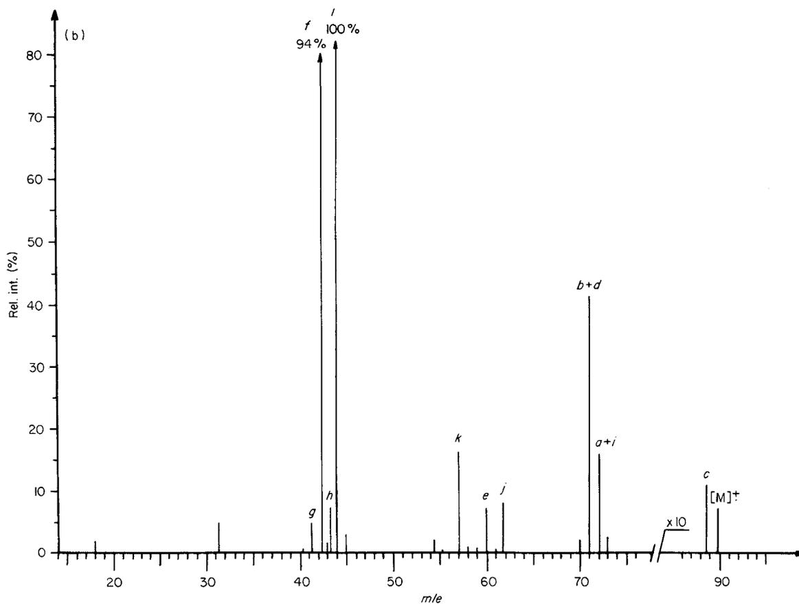
Figure 1. Mass spectra of 1,4-butanediol (1): (a) at 70 eV; (b) at 12.5 eV.
