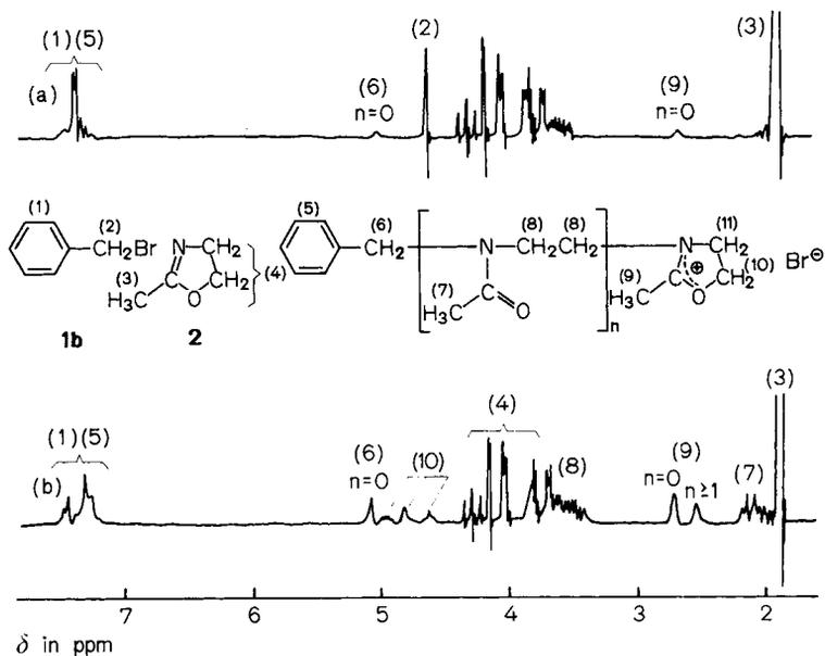
Fig. 3.  $^1\text{H-NMR}$  spectra of the polymerization system of **2** initiated by benzyl bromide (**1b**) in  $\text{CD}_3\text{CN}$  at  $35^\circ\text{C}$ . (a): after 2 min; (b): after 93 min
