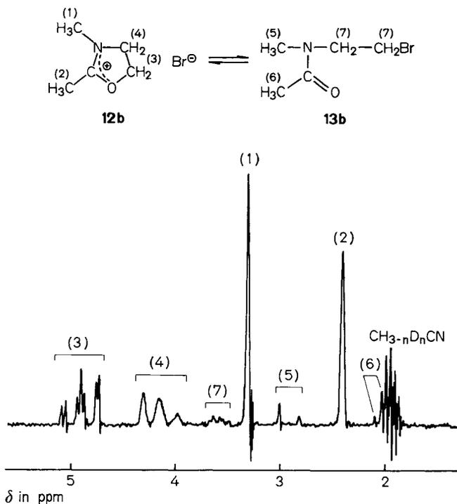
Fig. 5. <sup>1</sup>H-NMR spectrum of **12b** at 35°C in CD<sub>3</sub>CN
