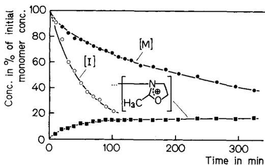
A kinetic analysis was made according to Eqs. (1)–(3) (Tab. 1). From the  $k_i$  values at  $40^\circ C$  (Tab. 1) it results that **1b** reacts 130 times faster with **2** than **1a**. The propagation rate of the system initiated with **1b** is 40 times faster than that of the system initiated with **1a**.
