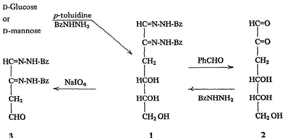
The reaction is illustrated by the preparation of 3-deoxy-D-*erythro*-hexos-2-ulose (2) as follows: a solution of D-glucose (2.5 g), benzoylhydrazine (3.2 g), and *p*-toluidine (1 g) in ethanol (50 ml), water (10 ml), and acetic acid (0.5 ml) was boiled
