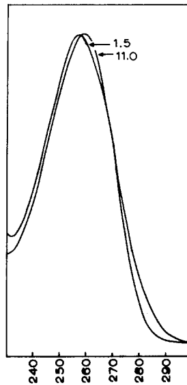
Fig. 3 Ultraviolet spectra at pH 2.5 and 11.0 of an unidentified nucleoside isolated from peak 2 of Fig. 2.
