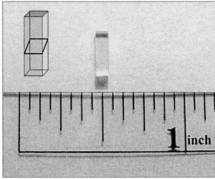
Fig. 1. YAG bicrystal specimen (boundary not visible) with schematic showing the boundary orientation relative to the surface.
