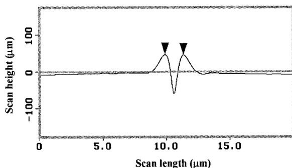
Fig. 2. Typical grain boundary groove, measured by atomic force microscopy. Note the symmetrical shape of the boundary.
