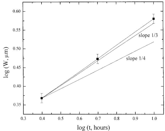
Fig. 3. Groove peak-to-peak distance,  $W$ , plotted as a function of time,  $t$ , for YAG heat-treated at 1600°C.
