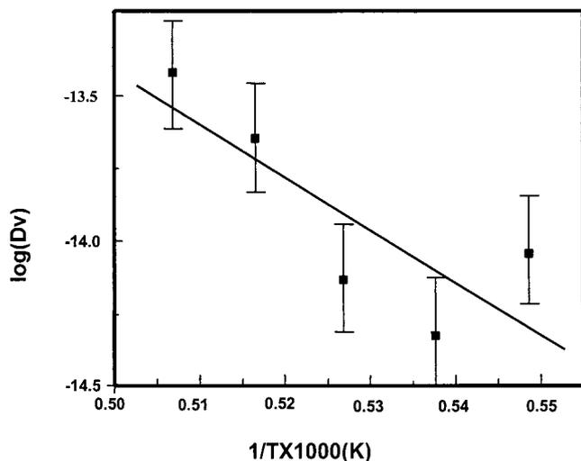
Fig. 4. Diffusion coefficients of YAG as a function of temperature calculated from grain boundary groove measurements.
