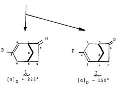
a (i) Obtained by resolution of the quinine salt from methanol (For a less efficient resolution see J. A. Berson and D. A. Ben-Efraim, J. Am. Chem. Soc., 81, 4083 (1959).); (ii) LDA; (iii)  $O_2$ ; (iv)  $Na_2SO_3$ ; (v)  $H_3O^+$ ; (vi)  $LiAlH_4$ ; (vii)  $NaIO_4$ .
