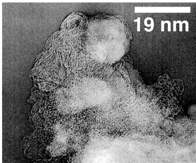
FIG. 6. HRTEM micrograph of another spot of the carbon of Leoville. This spot contains four microcrystals with parallel lattice fringes. These show  $d$ -spacings of 0.25, 0.29, and 0.50 nm.
