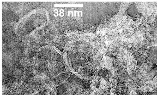
FIG. 4. Detail of a HTREM micrograph (inverted) of carbon from Vigarano. These structures may be carbon sacs similar to the "graphitic hollow calabashes" of Wang and Yin (1998). These could have formed by the pyrolysis of oxygen- or sulfur-bearing hydrocarbon polymers (Oberlin, 2002). They could contain noble gas atoms. The structures in area (b) of Fig. 2a in the Allende carbon appear to be similar. The areas not shown here were rich in carbon-black like carbon spheres.
