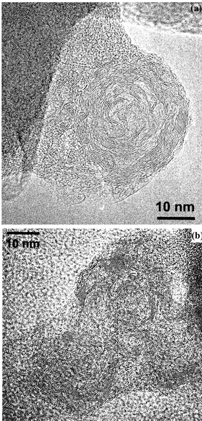
FIG. 3. (a) HRTEM micrograph of an apparently closed carbon structures from Allende sample AQ5. Notice the apparent internal voids in which noble gas atoms could be trapped. (b) A field of several onion-like particles. Such and similar structures occur in the samples from all three meteorites but involve no more than an estimated 10% of all carbon.
