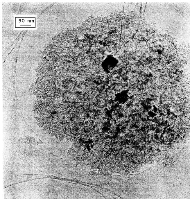
FIG. 1. HRTEM micrograph of a portion of the AQ1 particle of the Allende meteorite. Most of the sample consists of elemental carbon. The dark, blocky areas were identified as chromite grains or crystals by EDX analysis. This material was used for the microscopy study, results of which are presented in the following figures.
