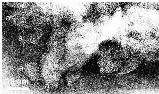
FIG. 5. HRTEM micrograph of carbon from the Leoville meteorite. This sample is rich in carbon spheres (a).
