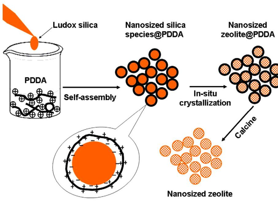
Fig. 4. Schematic diagram for the synthesis of MCM-22-NZ by the facile strategy combined self-assembly with in-situ crystallization.
