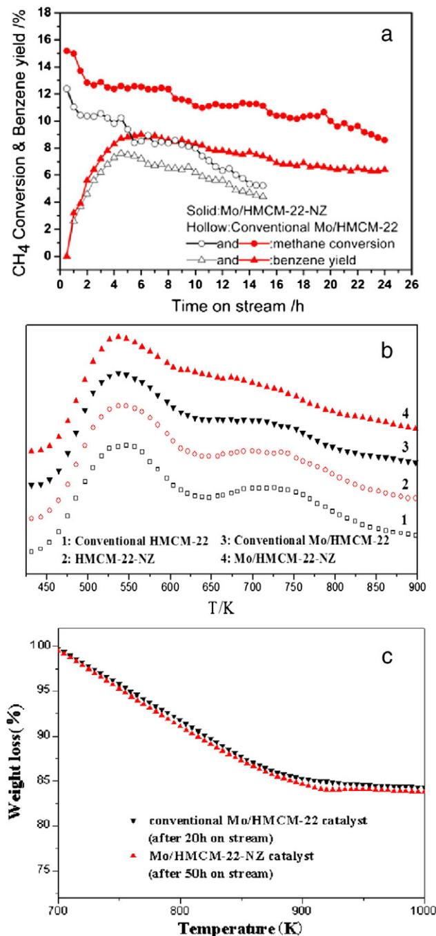
Fig. 5. The catalytic performance comparison for Mo/HMCM-22-NZ catalyst and conventional Mo/HMCM-22 catalyst in MDA reaction (a),  $\text{NH}_3$ -TPD spectra of the different catalysts (b), and TG profiles of the coked catalysts (c).
