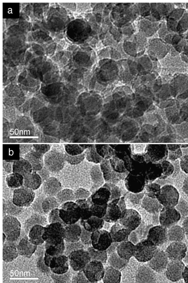
Fig. 3. TEM images of the synthesis colloids without PDDA (a) and with the presence of PDDA (b).
