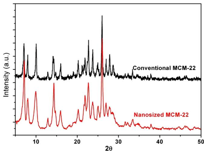
Fig. 1. XRD patterns of the nanosized and conventional micro-sized MCM-22 zeolites.
