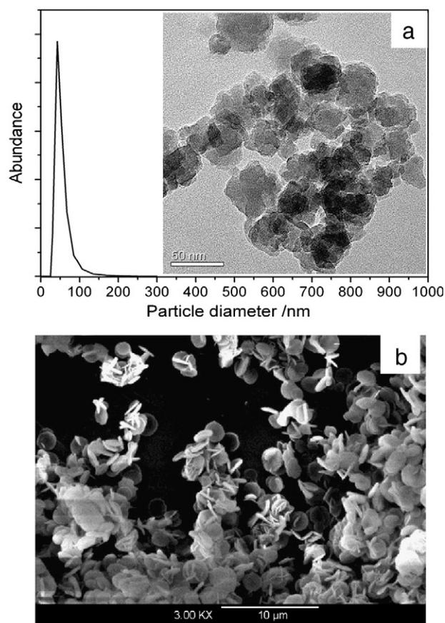
Fig. 2. Particle size distribution determined by DLS (a) and the corresponding TEM image of the MCM-22-NZ (inset figure in a), and SEM image of the conventional micro-sized MCM-22 zeolites (b).
