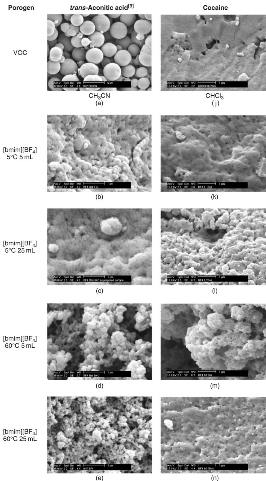
**Fig. 2.** SEM images of MIPs prepared using different porogens, temperatures, and volumes. (a)–(i) *trans*-aconitic acid MIPs, (j)–(r) cocaine MIPs.
