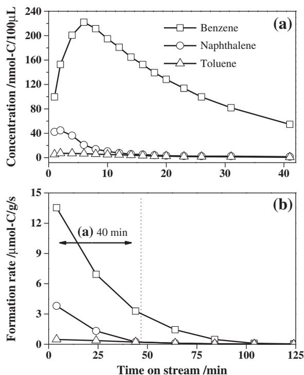
Fig. 4. Time dependences of the benzene formation activity of 5% Mo/HZSM-5 in the methane dehydroaromatization at 1073 K and 10,000 mL/g-cat/h, (a) measured in the proposed approach and (b) measured using the conventional on-line analysis method.
