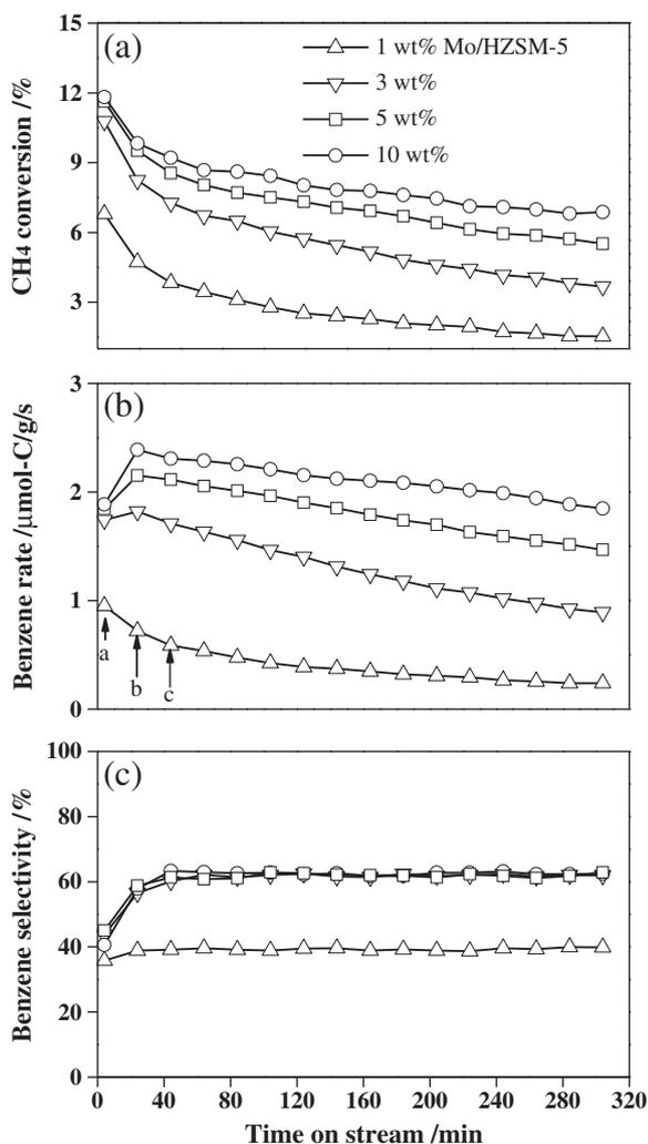
Fig. 3. Effect of Mo loading on the catalytic performance of Mo/HZSM-5 in the methane dehydroaromatization at 973 K and 3500 mL/g-cat/h, evaluated using conventional on-line analysis method.
