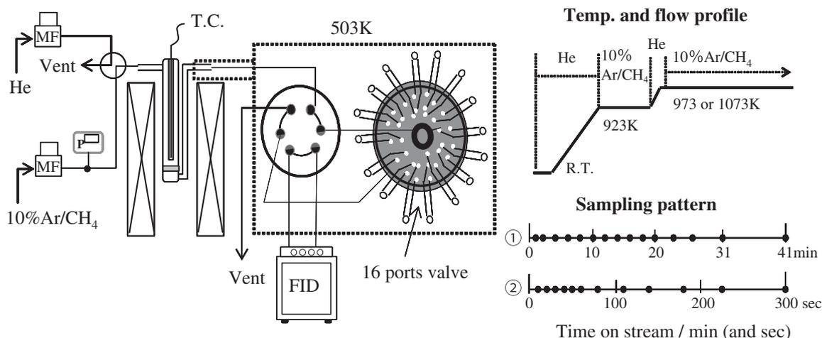
Fig. 1. The schematic of experimental set up, temperature and flow profile and two sampling patterns used.
