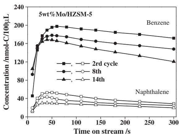
Fig. 5. Variations of outlet benzene and naphthalene concentrations with time in the 5 min CH<sub>4</sub> exposures of three different cycles of a 5 h periodic 5 min CH<sub>4</sub>-10 min H<sub>2</sub> switching test at 1073 K and 20,000 mL/g-cat/h.
