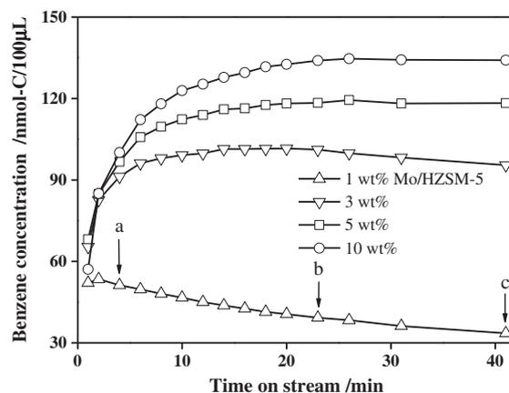
Fig. 2. Variation of outlet benzene concentration with time in the catalytic methane dehydroaromatization at 973 K and 3500 mL/g-cat/h, measured in the proposed approach.
