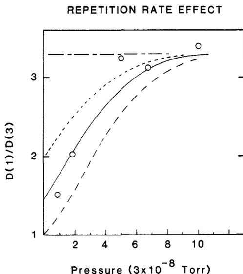
**Figure 4.** Ratio of dissociation at pulse rates of 3 and 1  $s^{-1}$ . Calculated curves are shown for assumed radiative rates of 0 (---), 1.5 (—), and 3 (— —)  $s^{-1}$ , as well as the cascade-model prediction (- · -) for radiative rates faster than 3  $s^{-1}$ .
