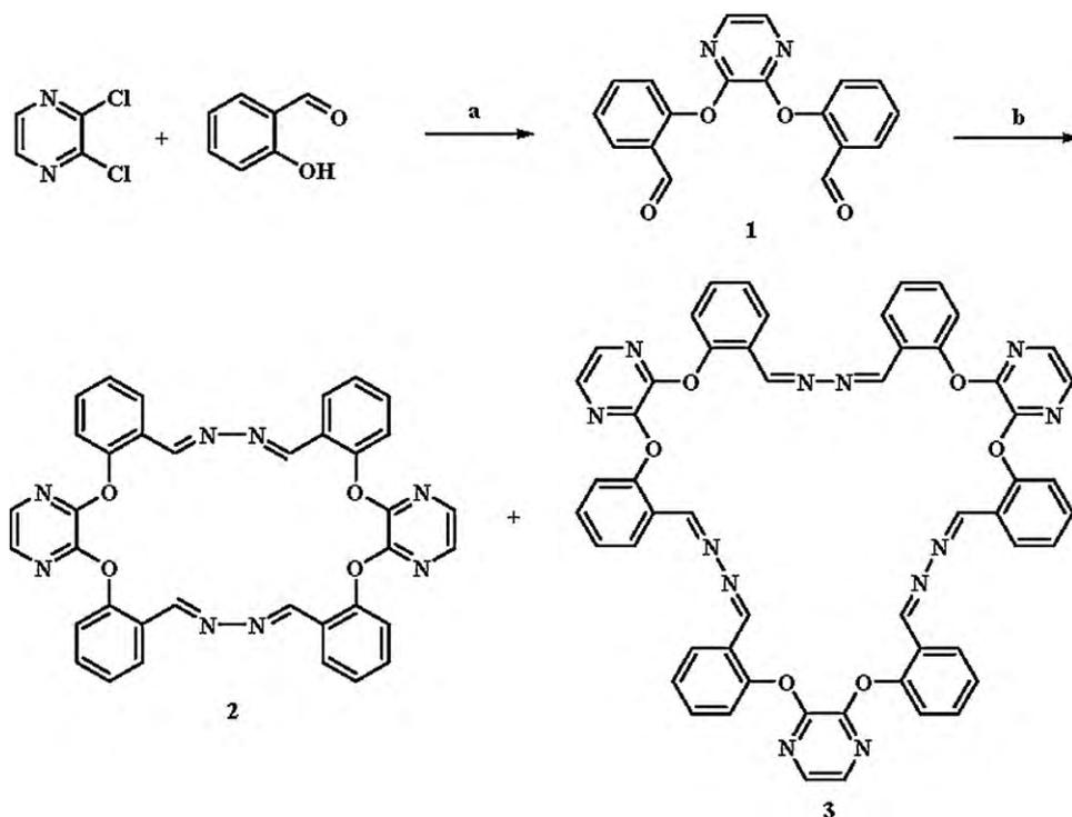
Scheme 1. Reagents and condition: (a)  $K_2CO_3$ , DMF, reflux, 12 h; (b) hydrazine hydrate, methanol, 24 h.
