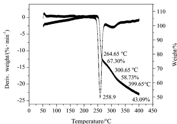
**Figure 2** TGA curve of DTZAF.
