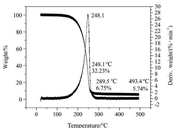
Figure 4 TGA curve of HATZF.
