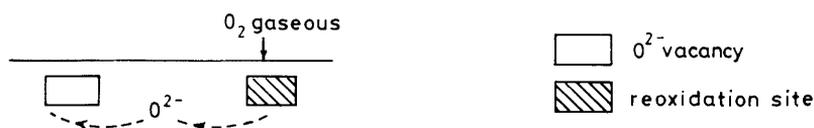
In view of this mechanism, the rate constants involve a catalyst in a partially reduced state during the catalysis. Under steady-state conditions, each reactant mixture produces a given vacancy concentration in the underlayers of the oxide. These vacancy concentrations lead to the observed structural modifications, probably due to distortion of the initial unit cell.
