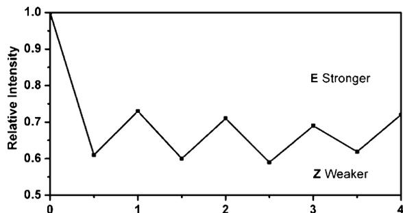
**Figure 3.** Changes in fluorescence intensity at 556 nm (excited at 345 nm) for  $\text{CH}_2\text{Cl}_2$  solution of protonated **E1** on alternating irradiation at 254 and 365 nm for four complete cycles.
