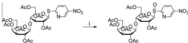
**Scheme 2.** Oxidation procedure for the synthesis of GP6. Reagents and conditions: (i) *m*-CPBA,  $\text{CH}_2\text{Cl}_2$ ,  $0\text{ }^\circ\text{C}$ .
