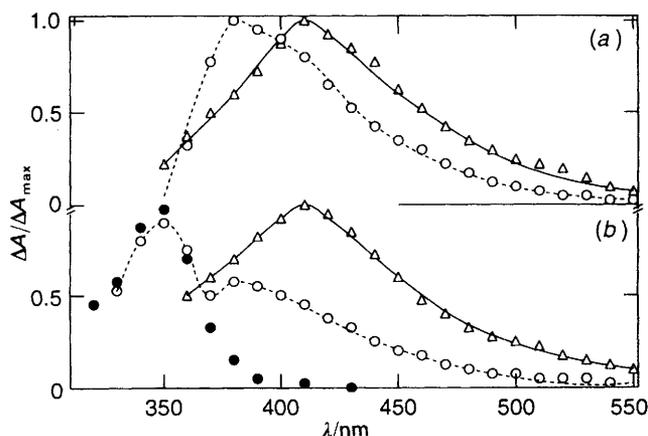
Fig. 4 T-T absorption spectra of (a) *trans*-AS and (b) *cis*-AS in cyclohexane solution at room temperature at the pulse end (O) and after 0.5  $\mu\text{s}$  (●), and in MCH at  $-196^\circ\text{C}$  ( $\Delta$ ), 1  $\mu\text{s}$  after the pulse,  $\lambda_{\text{exc}} = 248$  nm
