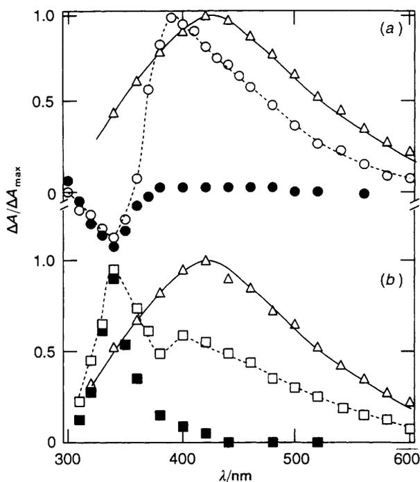
**Fig. 5** T-T absorption spectra of (a) *trans*-BS and (b) *cis*-BS in ethanol solution at room temperature at the pulse end (open circles and squares) and after 0.5  $\mu$ s (full symbols), and at  $-196^\circ\text{C}$  1  $\mu$ s after the pulse  $\Delta$ ,  $\lambda_{\text{exc}} = 248$  nm
