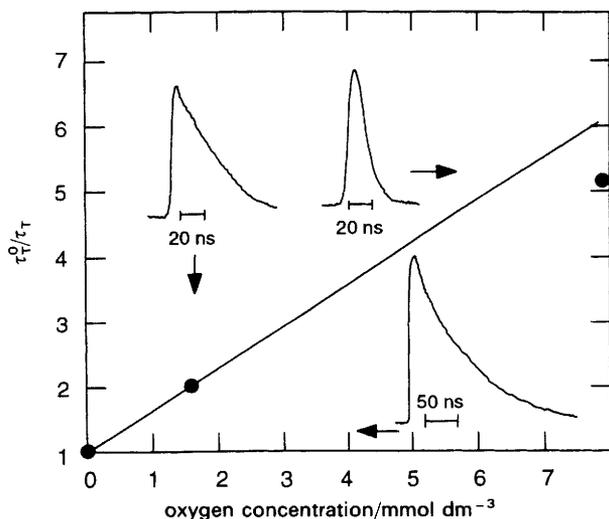
**Fig. 6** Plot of  $k_{\text{obs}}$  (normalized to  $\tau_T^0 = 75$  ns) vs. the oxygen concentration for *trans*-BS in acetonitrile. Insets: formation and decay of the triplet at 380 nm in argon-, air- and oxygen-saturated solution ( $\lambda_{\text{exc}} = 353$  nm).
