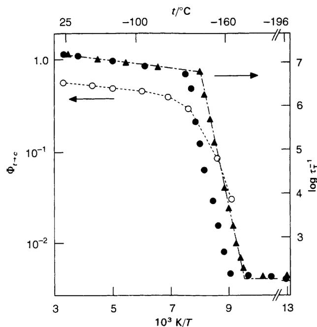
Fig. 3 Semilogarithmic plots of  $\tau_T^{-1}$  (full symbols,  $\lambda_{\text{exc}} = 248$  nm) and  $\Phi_{t \rightarrow c}$  (open symbols,  $\lambda_{\text{irr}} = 313$  nm) vs.  $T^{-1}$  for *trans*-BS in MTHF (triangles) and ethanol (circles)
