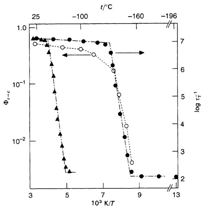
Fig. 2 Semilogarithmic plots of  $\tau_T^{-1}$  (full symbols,  $\lambda_{\text{exc}} = 353$  nm) and  $\Phi_{t \rightarrow c}$  (open symbols,  $\lambda_{\text{irr}} = 313$  nm) vs.  $T^{-1}$  for *trans*-AS in GT (triangles) and ethanol (circles)
