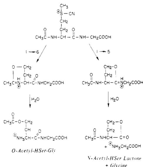
FIGURE 6: Diagram of the reaction pathway in which  $\text{CNBr}$  cleavage of Ac-Met-Gly yields *N*-acetylhomoserine lactone and glycine as major products and *O*-acetylhomoserine as a minor product.
