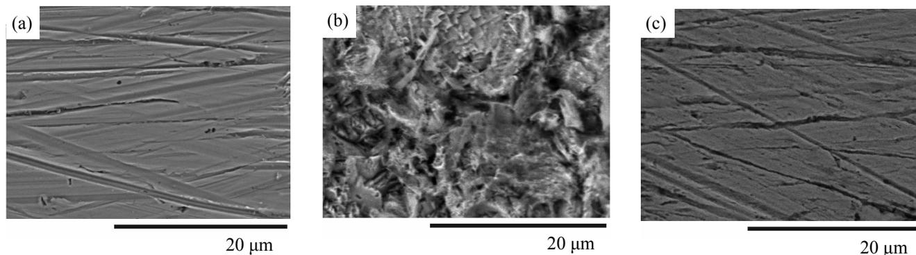
Soft steel plates: (a) pristine; (b) after 22 h incubation in corrosive medium; (c) after 22 h incubation in corrosive medium in the presence of 1 mg/L of salt **XIV**.
